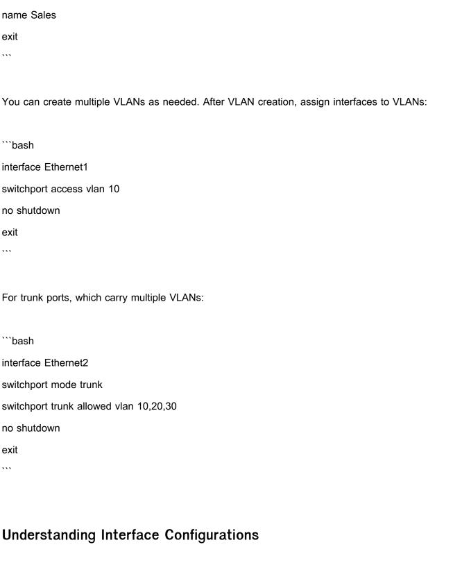
Arista switches support various interface types, including Ethernet, Port Channels, and Management interfaces. You can configure speed, duplex, and other parameters per interface:
